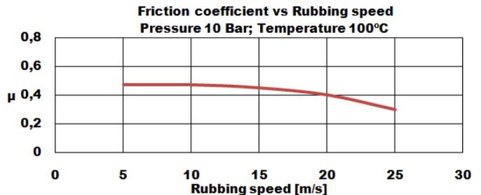
Rubbing speed, temperature and pressure are related. Changing any values will change other. The values shown represent typical conditions, but are not ultimate limits of the material.
